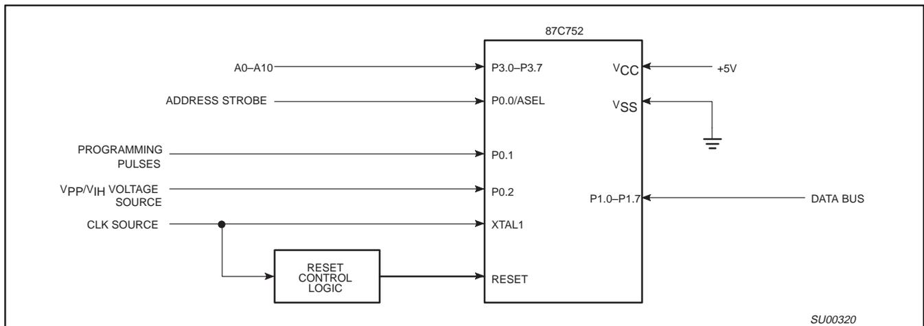
Figure 7. Programming Configuration
