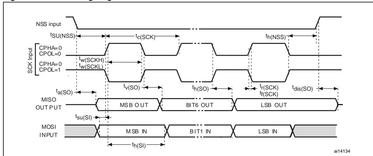
Figure 34. SPI1 timing diagram - slave mode and CPHA=1<sup>(1)</sup>
