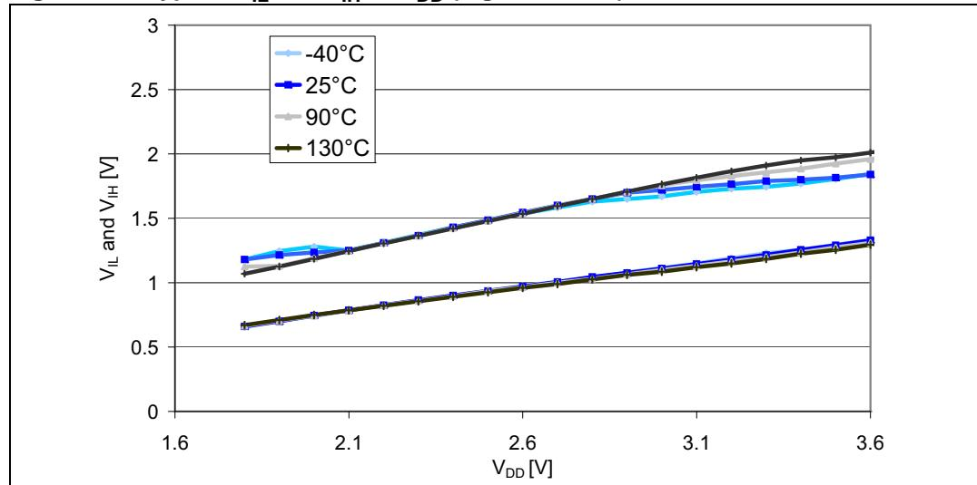
**Figure 21. Typical  $V_{IL}$  and  $V_{IH}$  vs  $V_{DD}$  (true open drain I/Os)**
