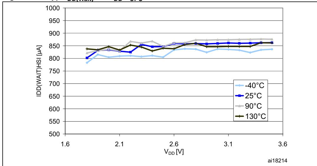
1. Typical current consumption measured with code executed from Flash memory.
