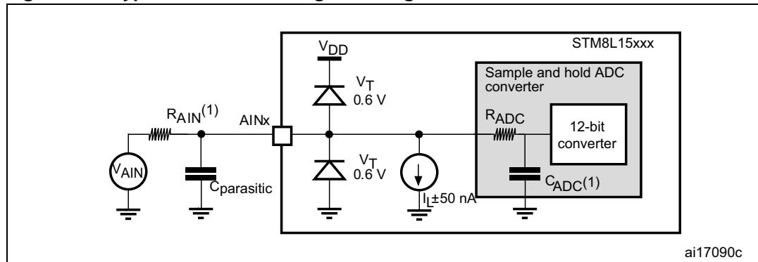
1. Refer to [Table 45](#) for the values of  $R_{AIN}$  and  $C_{ADC1}$ .
