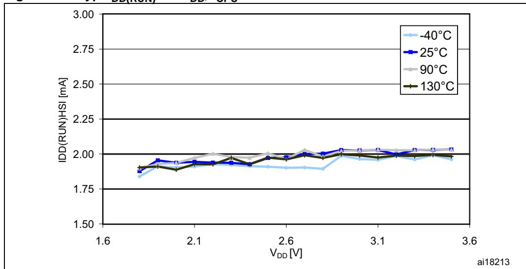
1. Typical current consumption measured with code executed from RAM
