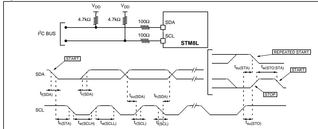
1. Measurement points are done at CMOS levels:  $0.3 \times V_{DD}$  and  $0.7 \times V_{DD}$
