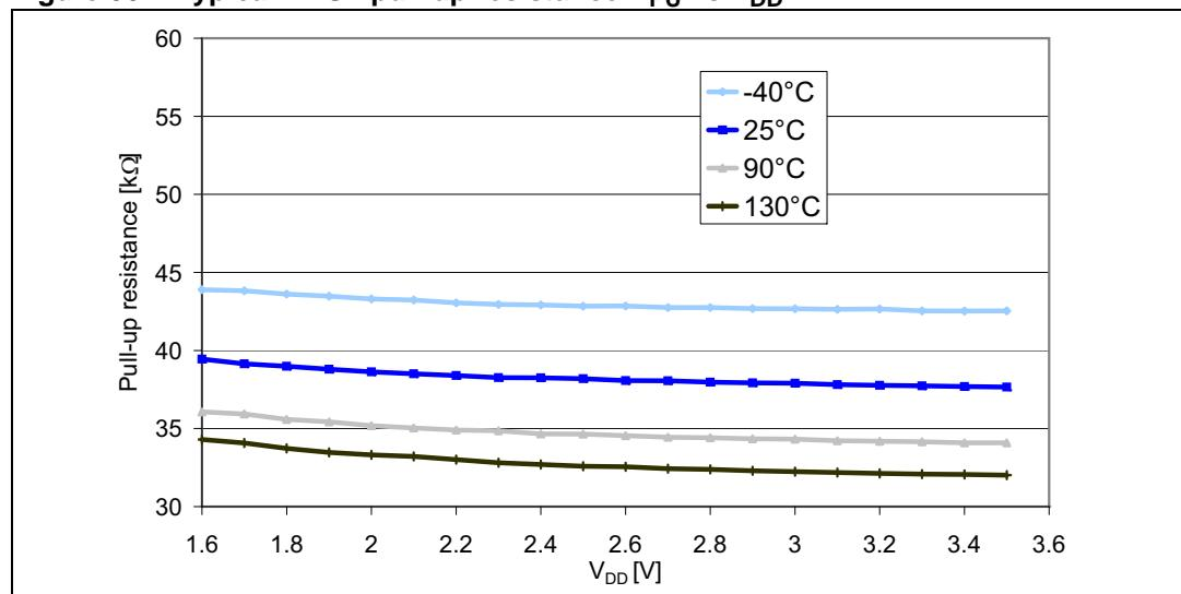
Figure 31. Typical NRST pull-up current  $I_{pu}$  vs  $V_{DD}$
