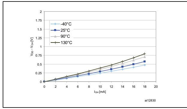
**Figure 29. Typ.  $V_{DD} - V_{OH}$  @  $V_{DD} = 1.8$  V (high sink ports)**
