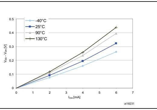
**Electrical parameters****STM8L151x2, STM8L151x3****NRST pin**
